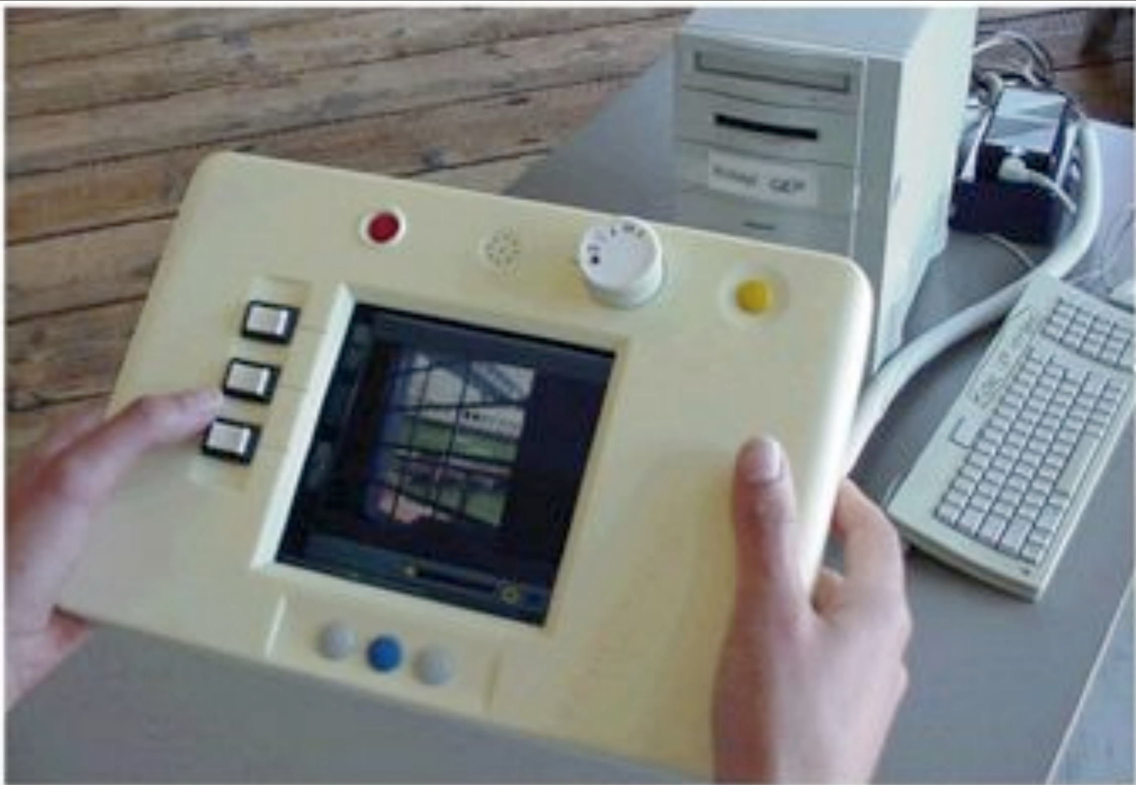
Figure 6: Digital camera interaction architecture prototype. The prototype used a desk-top computer's processing power to manipulate the dynamic qualities of the control system and screen behavior.
